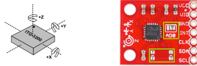
Fig. 4: Orientation of Axes of Sensitivity and Polarity of Rotation (Left) and Triple-Axis Digital-Output Gyroscope ITG3200 (Right)
